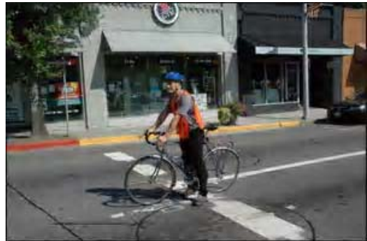
Bicyclist activates traffic signal by stopping over marking on Central Way at Lake Street
